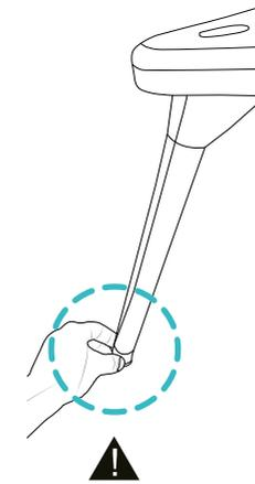
Screw the table legs into the holes on the underside of the table.
