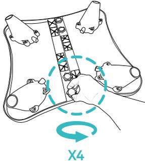
Connect the table plates together using 4 bolts.
